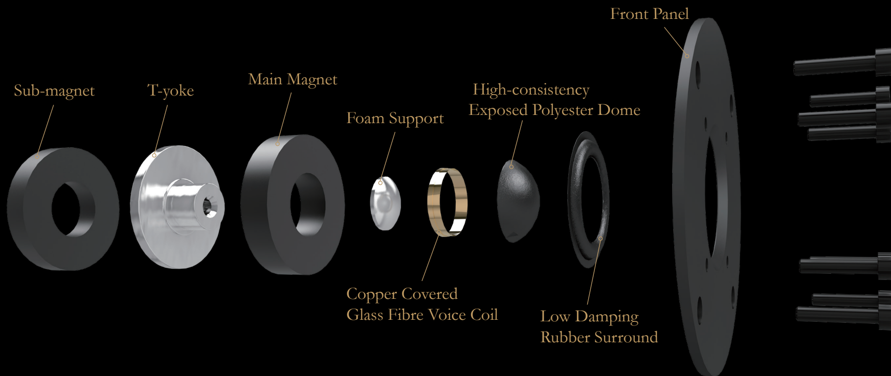
ABOVE: Exploded technical diagram of the Windsor series tweeter
